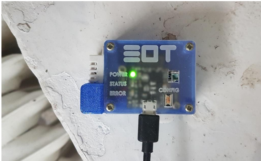
Figure 62: EOT sensor for temperature measurements, installed in Co-Working 02, south-wing
